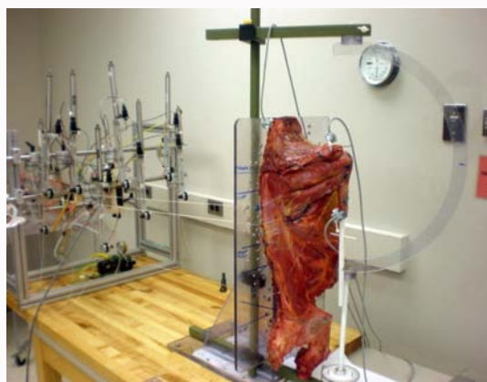
Figure 1: Novel shoulder model with a full hemibody fixed to hard block that has multiple holes, which allow the passage of cords from different muscle parts to pulley and pistons to attempt to replicate the normal shoulder muscle function.
